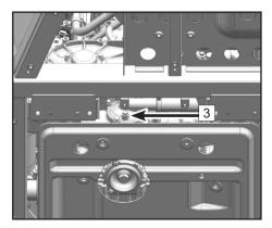
9. During filling coolant, unscrew the coolant drain bolt to release residual air inside the coolant hose until only fluid flows out, then screw back in and tighten the drain bolt.
